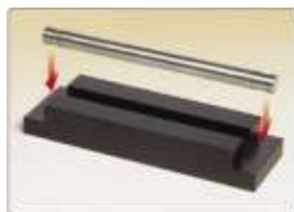
• Spacer bar and welding jig used during strain gage installation.
