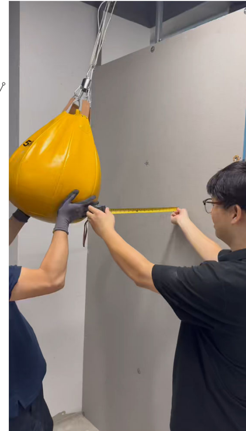
Figure 2 – Impact on vertical assembly h = drop height; L = length rope; \alpha = 65°
